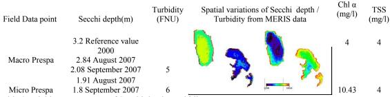
Table 2. Field measurements of Secchi depth, Turbidity, Chl α, TSS used for assessing MERIS data.
